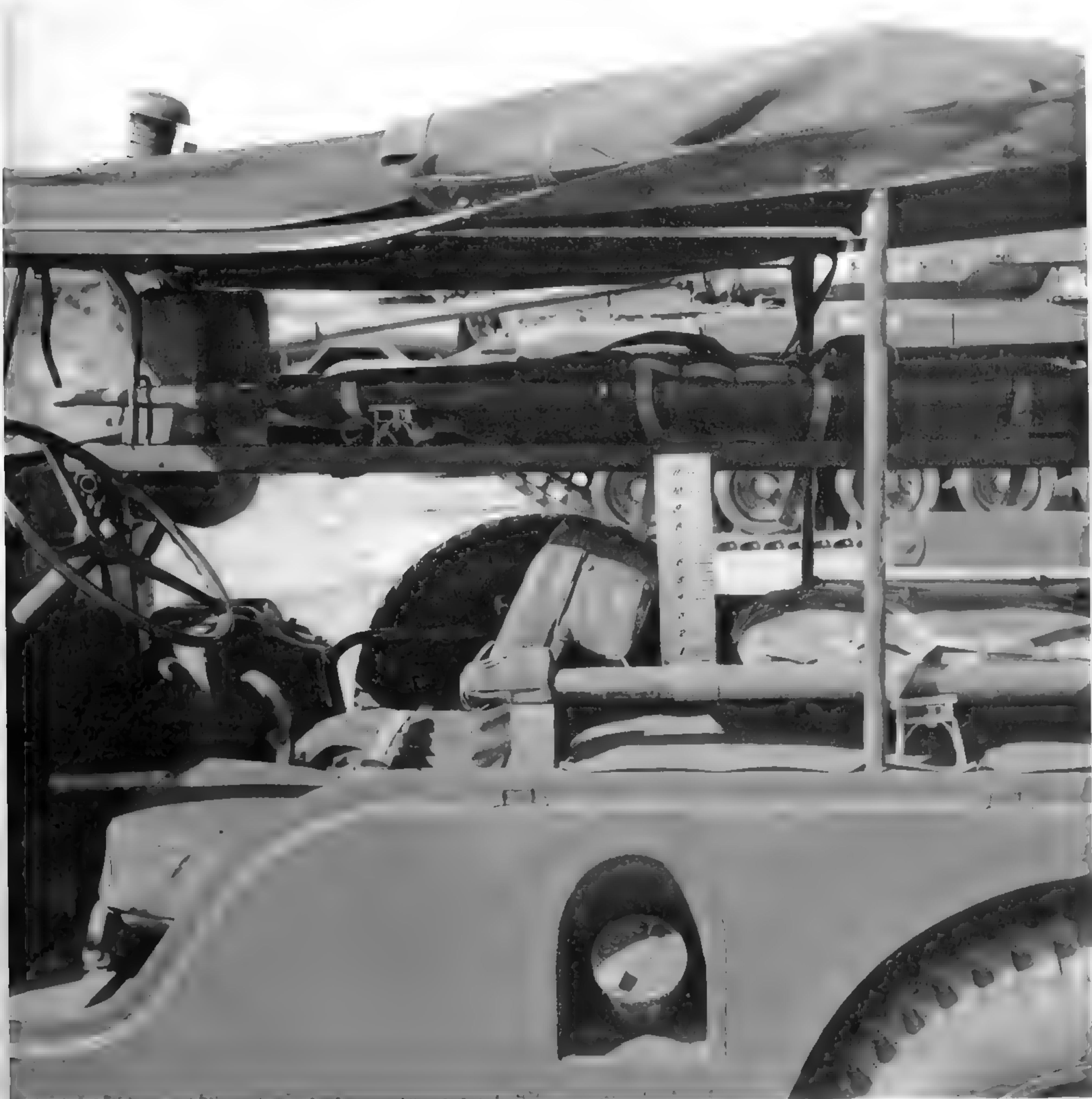
This view of the M170 shows how efficiently the limited interior space was utilized. A pad on the rear of the driver's seat protects the head of on patient, while the passenger's seat cushion has been hung from the windshield to protect the head of another patient. Also visible in this view is the interior-mounted spare tire and a 5-gallon gas can. No bracket for the gas can was installed, but footmen's loops were provided to secure it. (U.S. Army photo)
